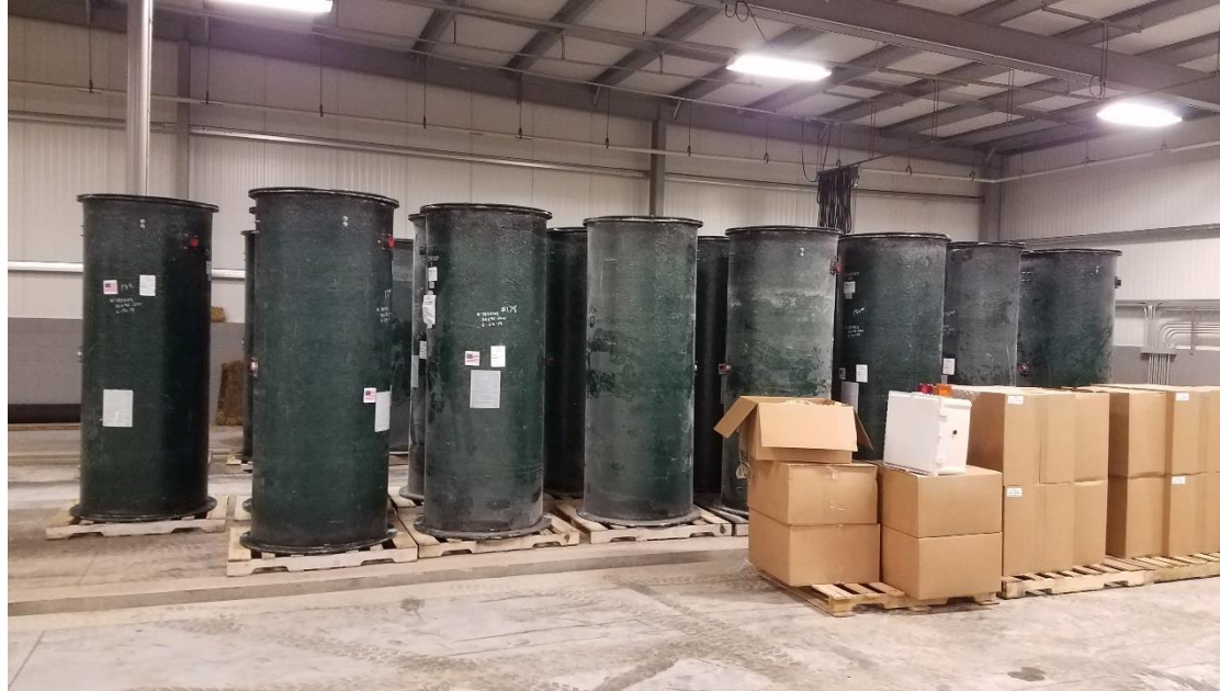
Grinder Pump Basins in Storage
